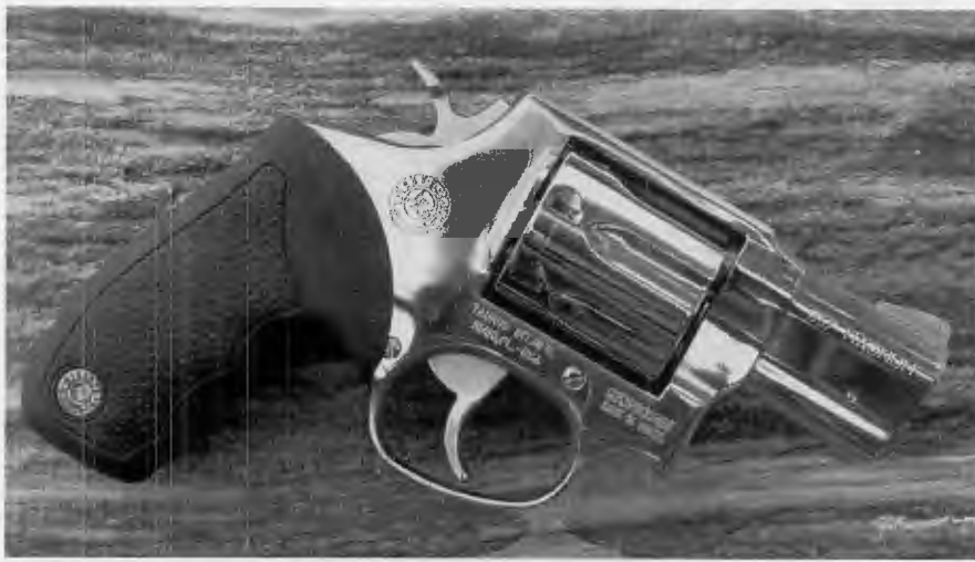
Taurus M617 .357 Magnum snubnose, right-side view. Note high-polish stainless steel finish, black neoprene-type grips and serrated ramp-type front sight. (right) Taurus key-lock safety system raises a pin and its shroud to impinge against the frame if someone attempts to roll the hammer rearward.
